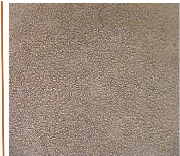
1R25 with DFF COPPER FOIL at 200X
