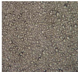
1R25 with TOCIII COPPER FOIL at 200X
