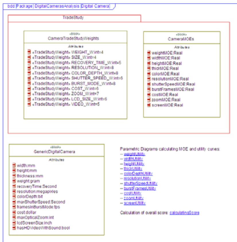
Figure 5: Digital camera BDD defining the relevant features of a digital camera for the trade study by the weights and the technical measures (MOEs). The hyperlinks on the bottom right side open the relevant parametric diagrams
