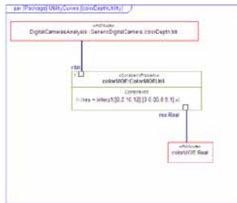
Figure 6: Parametric diagram for color depth utility curve
