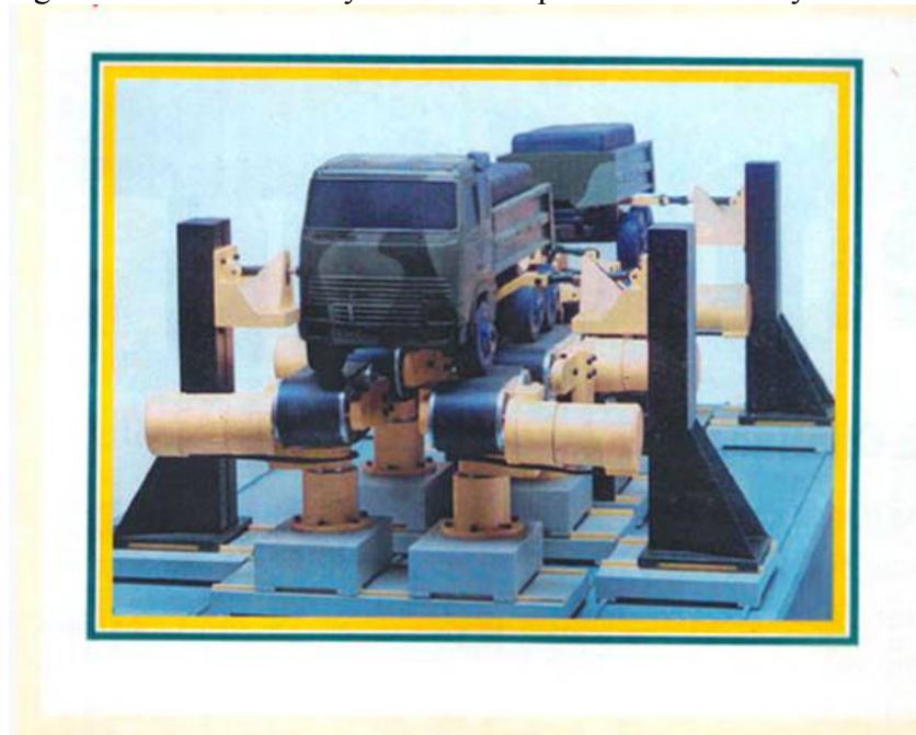
Fig. 13: Ground profile simulator at the Aberdeen Proving Ground [12]
